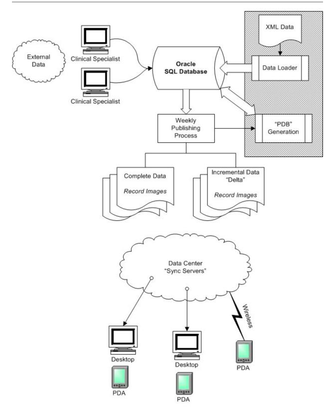
The gray area indicates the changes to the workflow for incorporating the new XML data.
